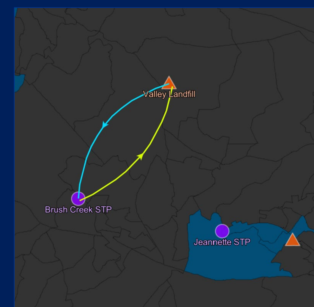
Figure 4. Movement of O&G wastewater from Valley Landfill to Brush Creek STP. Notably, solid waste is sent back to Valley Landfill, and from there material can leach back into groundwater.
